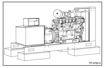
Figure 3-4 Four-Pad Mounting
